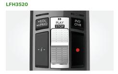
Slide-switch operation (fast forward, record/play, stop, fast rewind)
